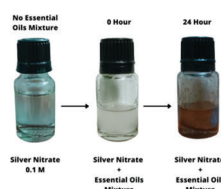
Figure 89.1. Depicts the essential oil - mediated silver nanoparticle synthesis. A metallic black was observed after 24 h of incubation at room temperature.
