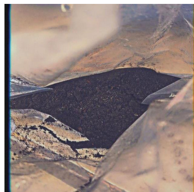
Figure 189.5. Activated biochar of Wodyetia bifurcata with HCl exposed to a temperature of 500°C using a muffle furnace, pulverized as microparticles.
